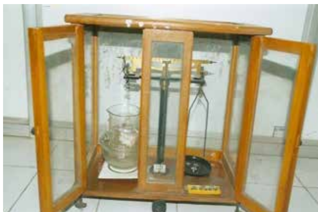
Fig 3: Bioadhesion testing apparatus
