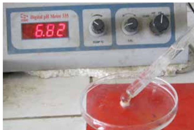
Fig 1: pH examination of buccal tablets using glass electrode
