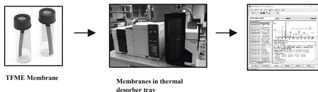
Figure 2: Desorption of TF-SPME membrane in GC-MS and identification of compounds by NIST library
