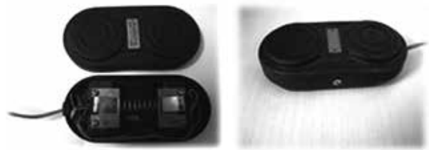
Figure 7: Foot Switch – (A) Inside; (B) Outside
