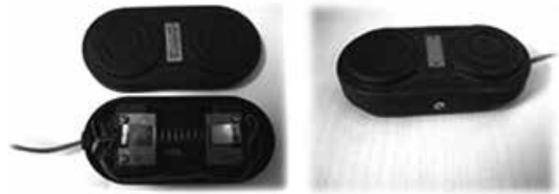
Figure 7: Foot Switch – (A) Inside; (B) Outside
