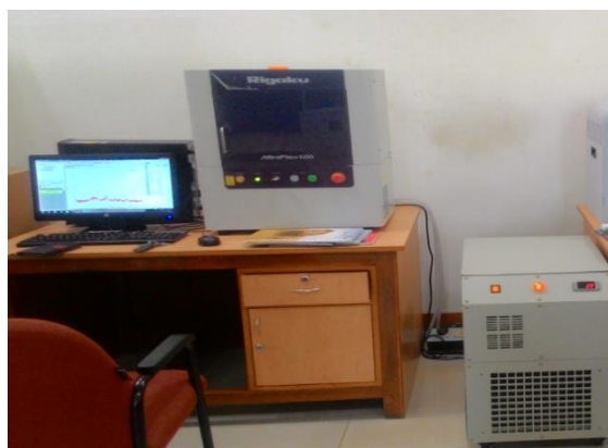
Figure 2: Powder XRD (Voltage-20-40V, Current-2-15mA along with chiller water circulation)
